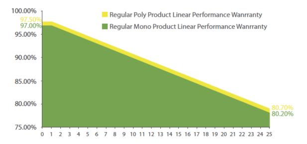
3). Double glass Poly product exhibits a power output no less than 97.5% of the nominal peak power specified on the respective datasheet or module label at STC within the first year from the "warranty start date", and power output declining by no more than 0.5% per year of the nominal peak power as specified on the respective datasheet at STC from the 2<sup>nd</sup> year to
