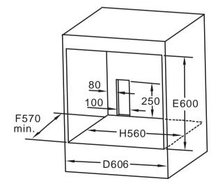
Remark:1.Only plus deviations are admissible for all dimension.2.The cabinet is not include the power switch or socket.
