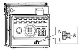
Disconnection from the supply may be achieved by having the plug accessible or by incorporating a switch in the fixed wiring in accordance with the wiring rules.
